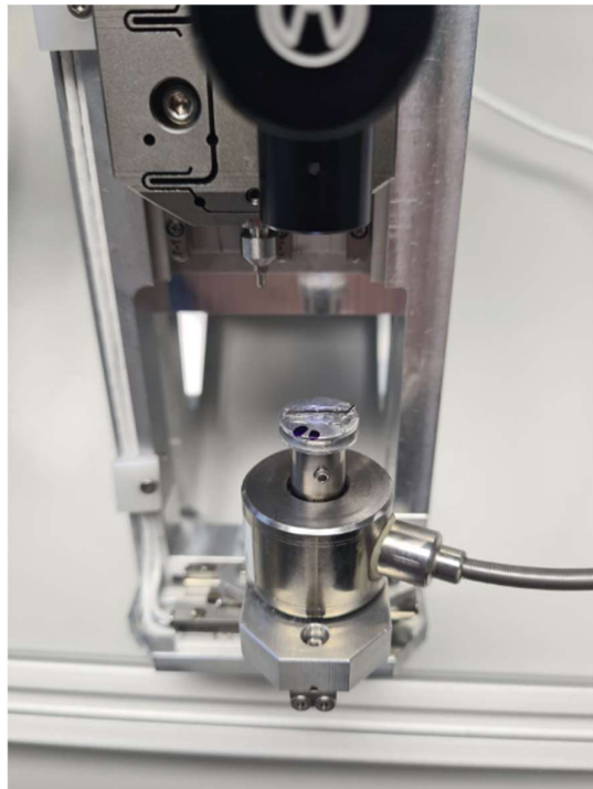
Fig. 10: Diffusion Bonded Joint sample mounted under the ASA in the microscope position
