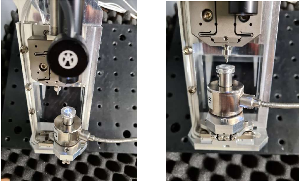
Fig. 4: Fused Silica (FS) sample mounted under the ASA in microscope position and indentation position
