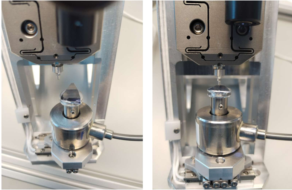
Fig. 12: Al-on-Si sample mounted under the ASA in microscope position and indentation position
